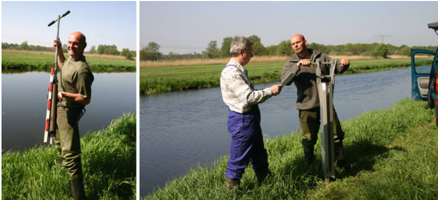
Fig. 8 Dutch sampler and Wardenaar sampler in use on peatlands and under semi-aquatic conditions. Both samplers are commercial products of the Eijkelkamp company, Giesbeek, The Netherlands
