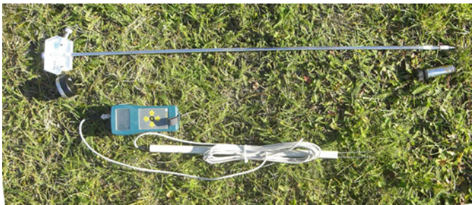
Fig. 3 Field tensiometer (Tensio 100 of UGT Muencheberg) and field TDR probe (Easy—Test, IPAN Lublin) may provide information rapidly on the soil water status
