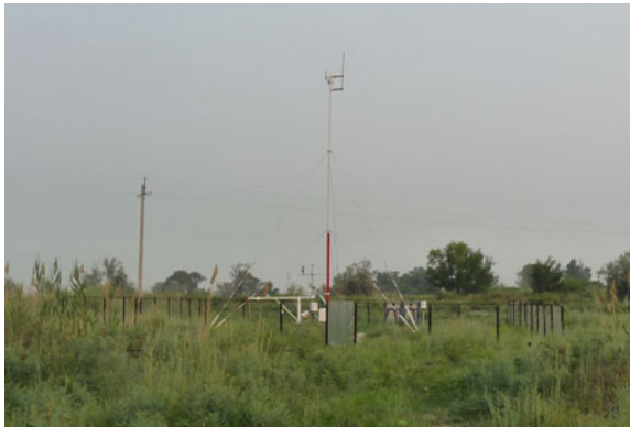
Fig. 29 Agri-environmental monitoring station in the meadows of the Ili river. Modern monitoring stations for agrometeorological and environmental data to calculate water, solute and gas exchange of soils and vegetation with the atmosphere are essential for modern research. Kazakh researchers from the Uspanov Institute of Soil Science and Agrochemistry plan to set up the first generation of such stations
