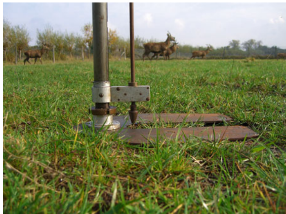
Fig. 2 Vertical penetrometer for testing soil strength on a red-deer pasture in the research station Paulinenaue, Germany
