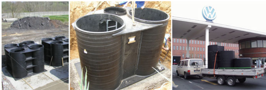
Fig. 4 Alternative designs of containerised PE-HD lysimeter stations (from left to right —4-fold, 2-fold and 1-fold lysimeter station during installation)
