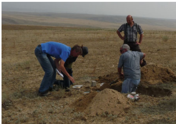
Fig. 4 Soil sampling for assessing soil quality and measuring soil hydraulic properties in a joint Kazakh-German project
