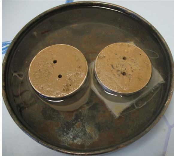
Fig. 2 Saturation of samples and tensiometer holes
